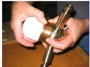
Expand the jig by rotating the two components in each hand so as to undo the threaded portion of the jig
