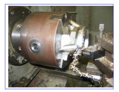
Machine face in two cuts to jig setting
