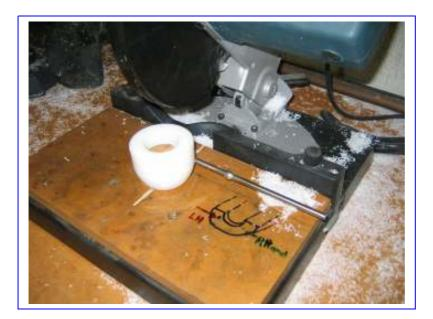
Split in two with cut off saw holding the tool still at right angles by maintaining alignment with the marks
