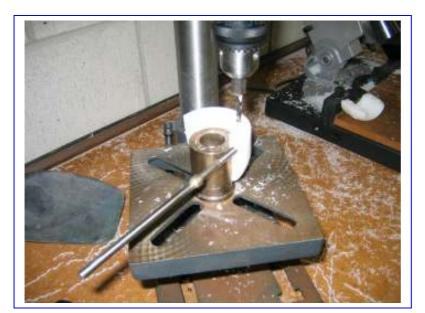
Mount on jig to bore and recess spring hole.
