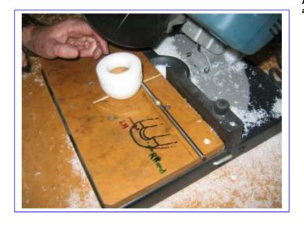
Align tool with mark to ensure cut is at right angles to bolt holes
