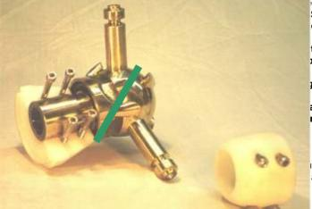
SS Pod with ¼" BSW ( = UNC ) thread inserted for Left d Prop as a guide to prevent subsequent interference S ¼" Screw at assembly time. [ Braze rod into head of et screw ]
