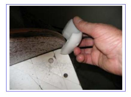
Grinding off the inner corners to enable easy assembly subsequent assembly.
