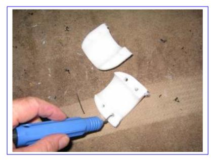
De-burr all the cut surfaces using a de-burring tool.
