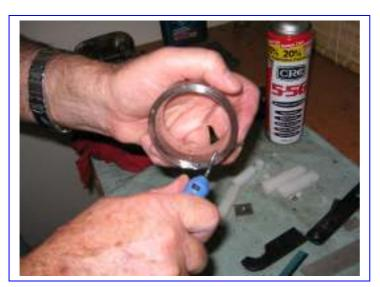
Deburr inside edge with deburring tool
