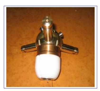
The jig is threaded and fits over the Boss to be expanded by unwinding the two halves until a snug fit between the blade carrier and the nose cone which is held manually in place
