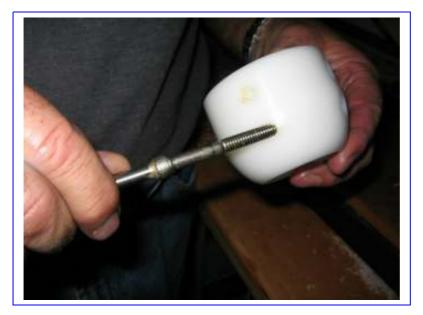
Insert the tool into the lower  $\ensuremath{^{1\!\!/4}}\xspace''$  UNC thread as shown.
