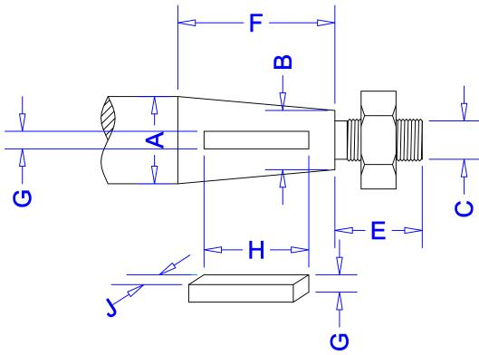
If shaft drive, please give the shaft/taper/key details below. If spline, please give the make and model.
